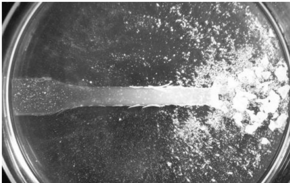
Figure 9 Organic solvent treatment evaluation of phase structure inclination material. Sample: modified epoxy resins containing 20 wt % of PES. Organic solvent (DMF) treatment: 23 h at 23°C.
